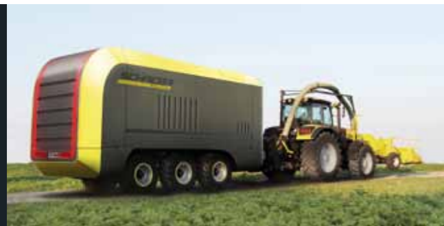
The mobile harvester Schaidler Pelletec D 8.0 Producing up to 8 tons of ready-for-use pellets per hour directly on the field.
